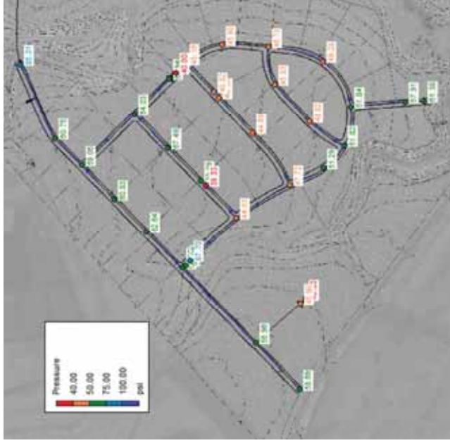
Figure 8- Residual Pressures with 2000 gpm Commercial Fire Flow
